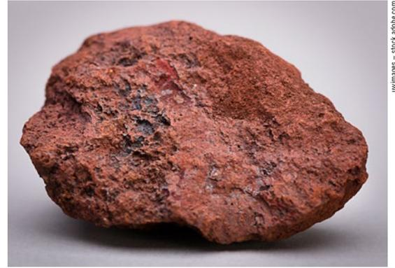
Hematite (also known as red iron ore) is a commonly occurring iron oxide (Fe<sub>2</sub>O<sub>3</sub>) with an iron content of up to 70%.
