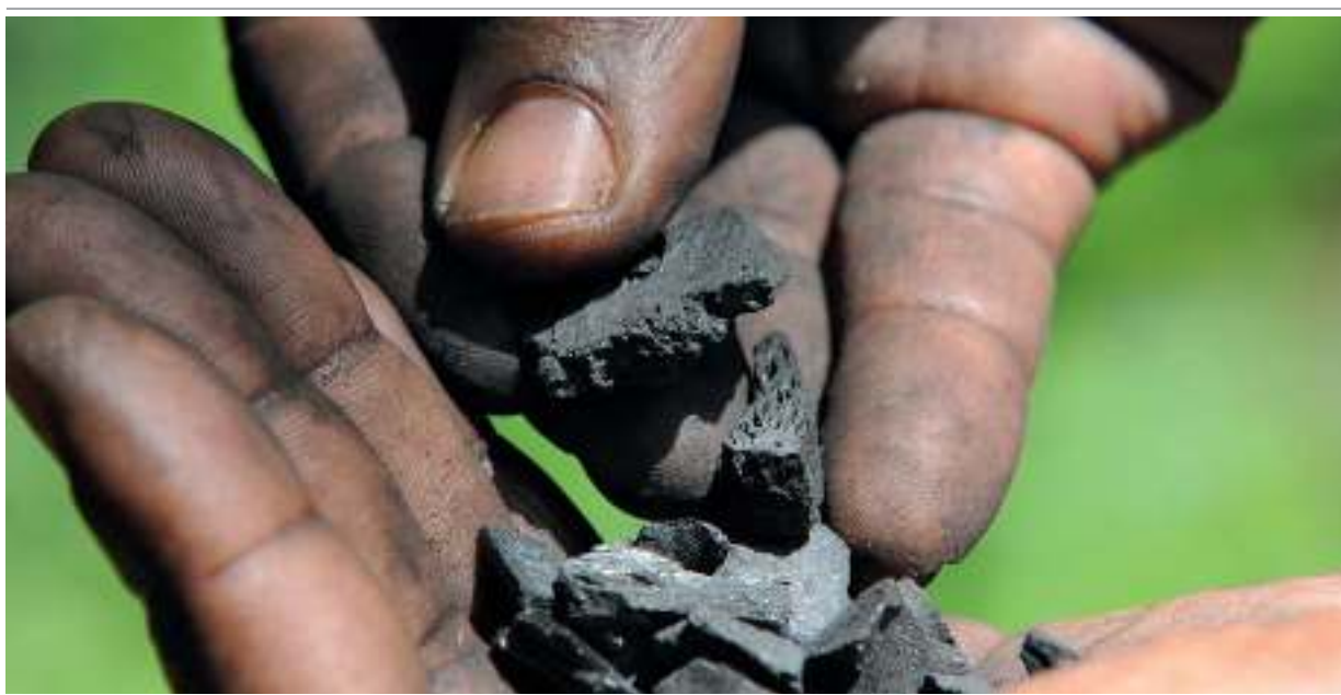
Biochar, the product of pyrolysed biomass
